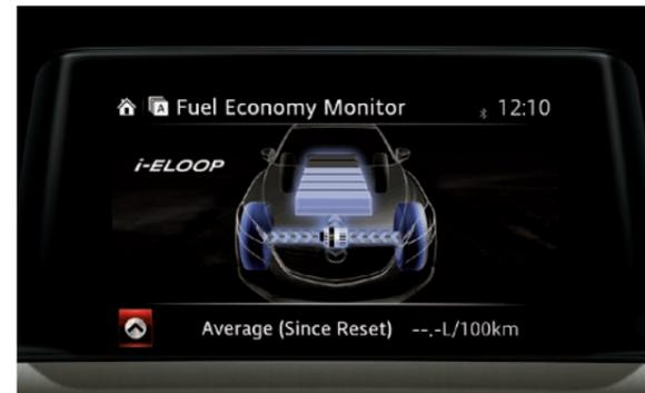
Mazda's i-stop idling stop system automatically shuts the engine down when you halt after braking. And the i-ELOOP regenerative braking system captures energy lost during deceleration, saving it as electrical power. Both technologies contribute to Mazda3's excellent fuel economy.
