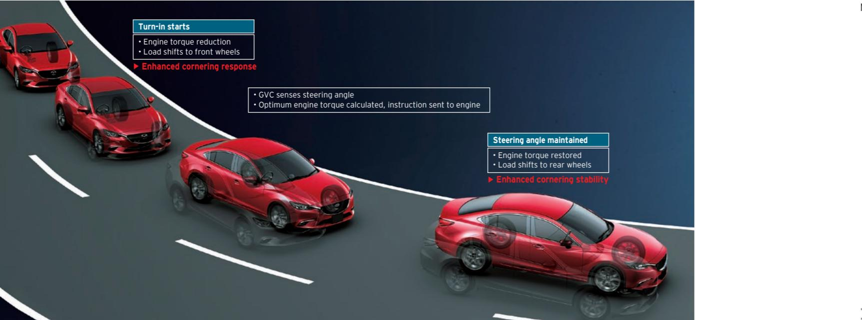
characteristics. GVC is a new approach to controlling vehicle dynamics that uses the engine to enhance chassis performance, and it gives Mazda vehicles even smoother transitions between G-forces in all driving scenarios.
